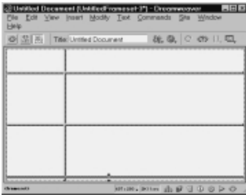
Figure 13.26 Click on the border of the unwanted frame, and drag it off the page. You'll get rid of both the frame and the border.
