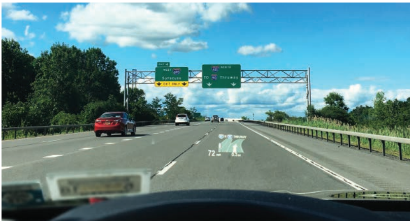
FIGURE 1.8 HUD. The driver's view of navigation using a head-up display featured in a BMW.
