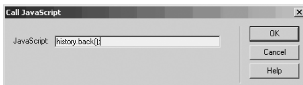
Figure 8.15 The Call JavaScript dialog box allows you to add custom scripts to your pages.
